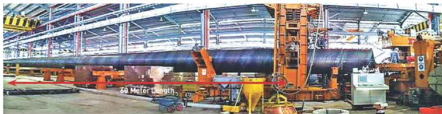
Pipe Manufacturing to 60m Length
