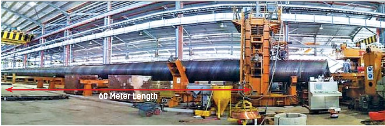
Pipe Manufacturing to 60m Length
