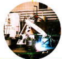
Robotic Welding Process (MIG) by Artificial Intelligent Robot.
