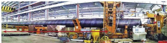
Pipe Manufacturing to 60m Length
